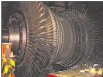
Steam Turbine LP Turbine
