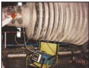
TOFD Test on Steam Turbine
