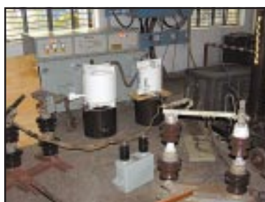
Discharge current test setup for series capacitors
