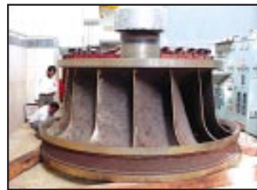
Runner of Hydro Power Plant
