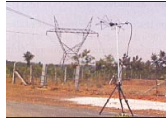
Interference measurements in progress near a HVDC Line
